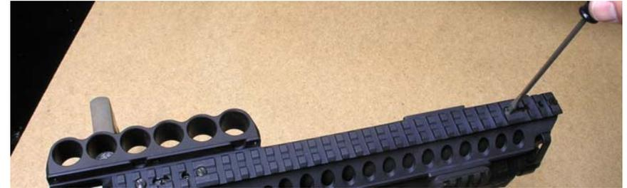
Now use the gold hex keys (blue in these photos) to fully tighten the M4 button head screws and the angled set screws.
