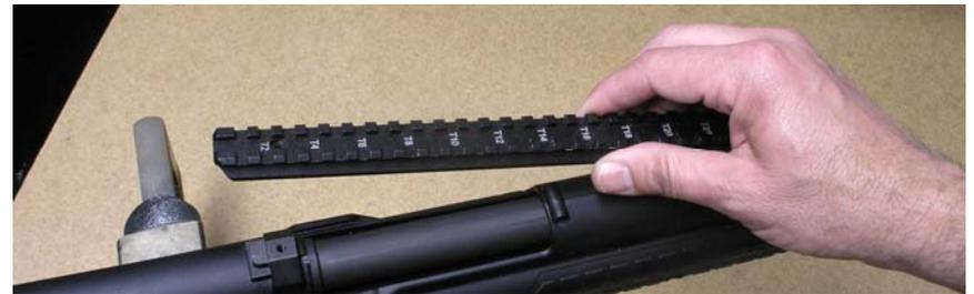
Behind the rear rail mounting pillar is a small plastic recoil lug. Remove this as well:
