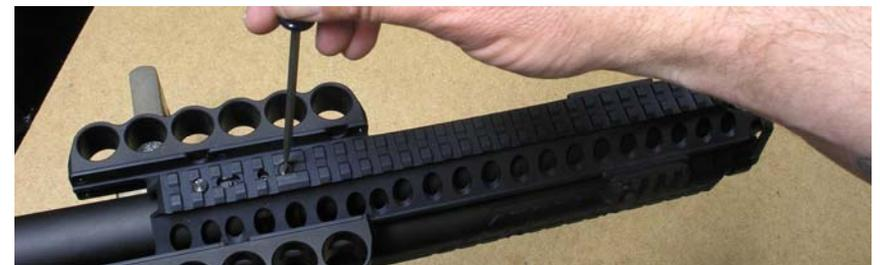
Once you have established that everything fits well together, we suggest you disassemble the SureShell Carrier and Rail for the Kel-Tec KSG and re-assemble it once again, putting a drop of blue Loctite on each threaded fastener.
