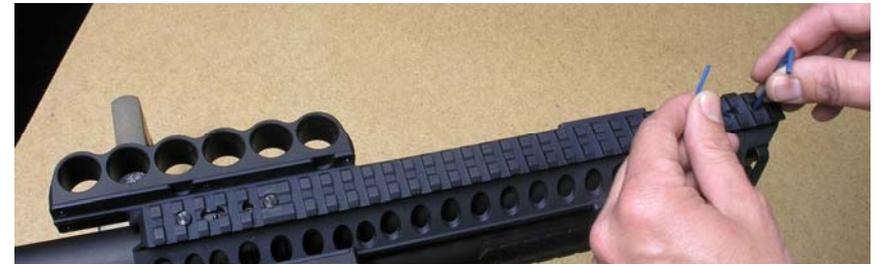
Finally, go back and re-tighten all four of the slotted top rail mounting screws.
