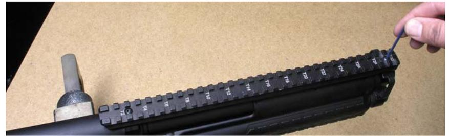
Once the screws are out, remove the rail:
