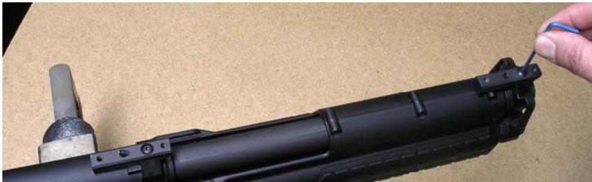
Place the SureShell assembly on the recoil blocks and secure it in place using the four slotted head screws and conical washers.
